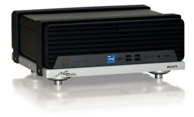
The HP Elite 800 G9 Small Form Factor (SFF) PC is marine type approved by most of the major international marine Classification Societies when it is installed in conjunction with our Mariner Kit MS2670.
